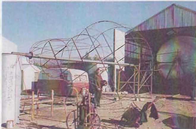
The gel coat has been applied to the apple in the shed whilst the frame work of the pear is pictured with Steve Bell in the foreground.
